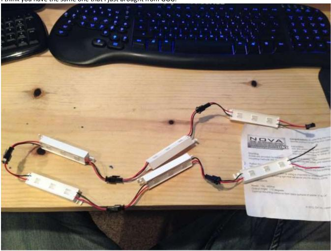
At the end of this string of LEDs you should see that there are two wires there. You can also see from the instructions (circled below) that the LED strip is 12v.
