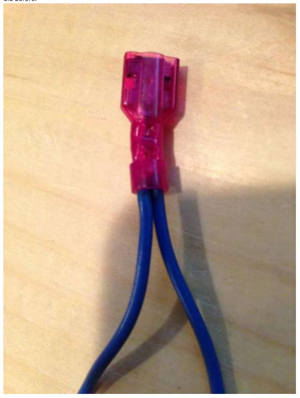
For the "ground" or "common" wire of your controls, which we will cover in greater detail later on, you will be daisy chaining a wire from one control to the next. The same ground wire will go to each and every switch you have. So they will go from button to button, to the switches on the joysticks, etc. So in the end, you will wind up with one wire with tons of disconnects on it, that will link together everything.
