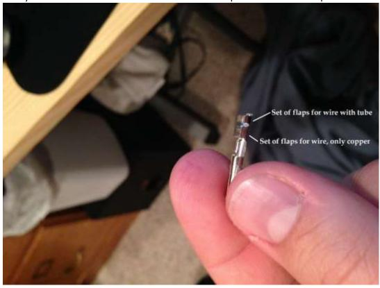
As you can see from the previous picture, one set of flaps you will be clamping around the stripped copper wire and the other you will be clamping down a little lower around the wire that still has the plastic casing around it.
