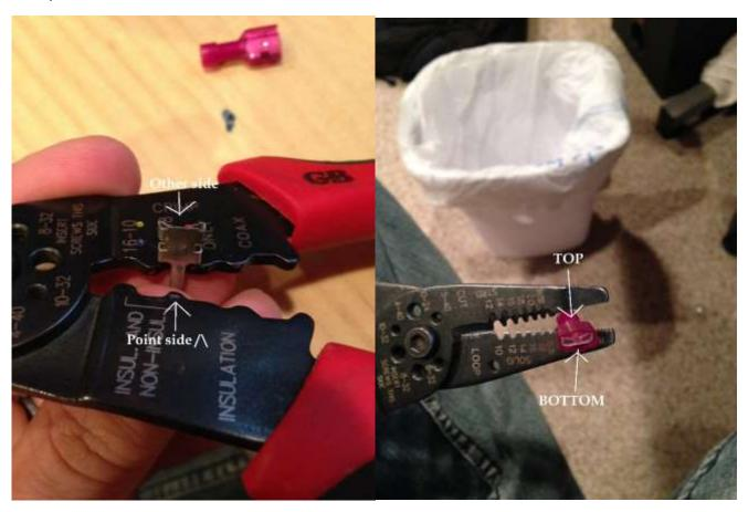
Now, once it's correctly held in place, clamp together the crimper tightly. You don't want to absolutely kill the thing, but you do want to press tightly so that it creates an indentation in the tube part:
