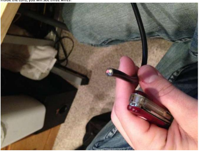
Use a small knife, or whatever method you want, but cut the casing around the three wires:
