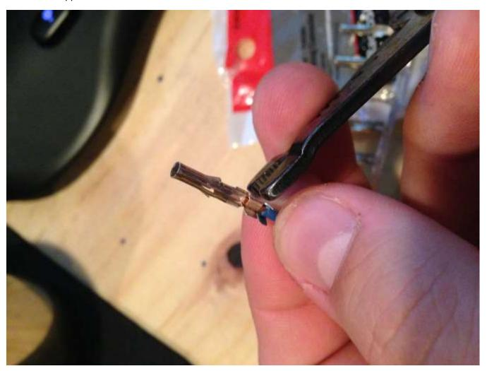
Next fold the other side of the flap over, right on top of the other one. Once both flaps are in place, just use the pliers to give the pair a good clamp, real tight, so that the flaps are very securely holding around the copper.
