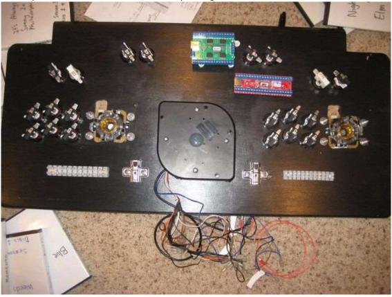
And here you can see it with all the wires attached. I tried to get it so that the wires sort of pointed in the same direction, so that I would have bunches of wires that I could zip tie together.
