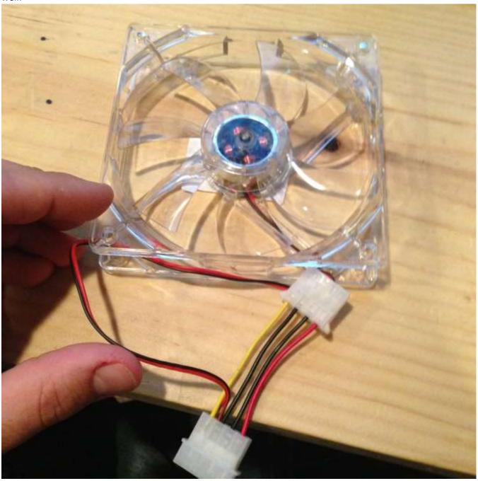
We're actually going to be cutting off that PC power connector, but before we do, we need to figure out if your fans are 5v or 12v. Take a look at the two wires coming off the fan, and look at where they tie into the PC connector power wires:
