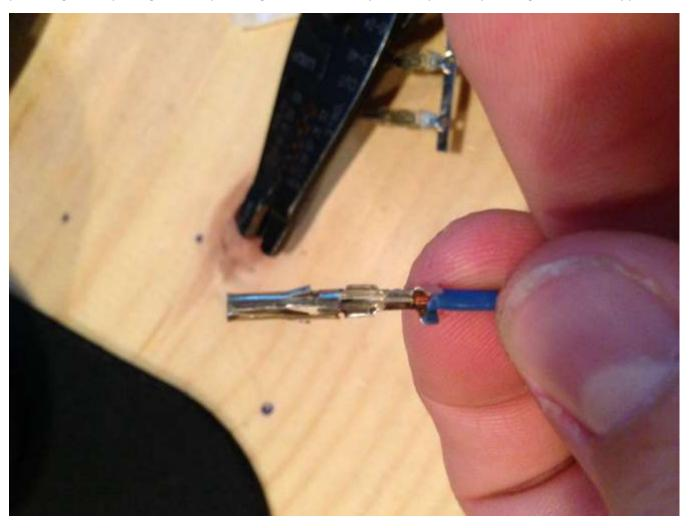
Next repeat this process for the bottom flaps that go around the wire that still has the casing on it. One flap first:
