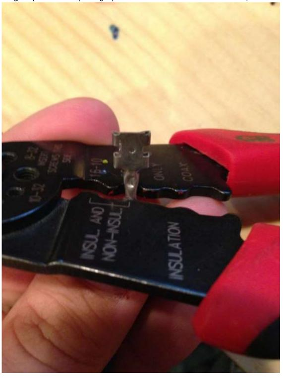
Next, move the crimper a little bit down and repeat on the bottom half of the tube, so that there are two crimps holding it in place:
