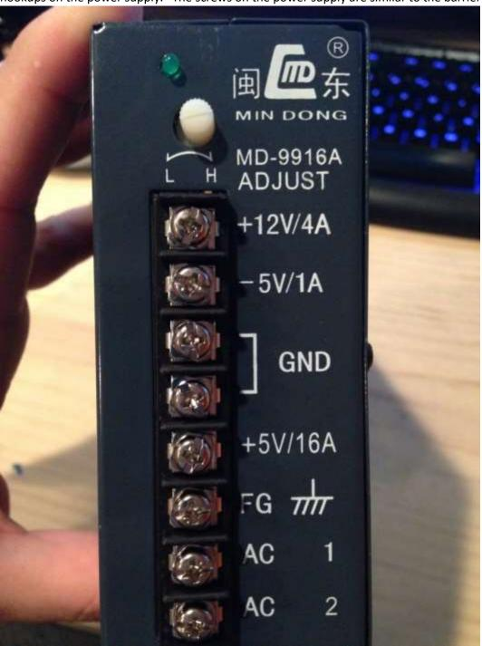
So you will be hooking up one wire to the +12V hookup, one wire to the +5Vhookup, and one to (one of) the ground hookups on the power supply. The wires you will be rigging up will then, if you haven't figured it out, have an O-ring on each side. Each wire will connect over from the three items I mentioned above over to their own barrier strip:
