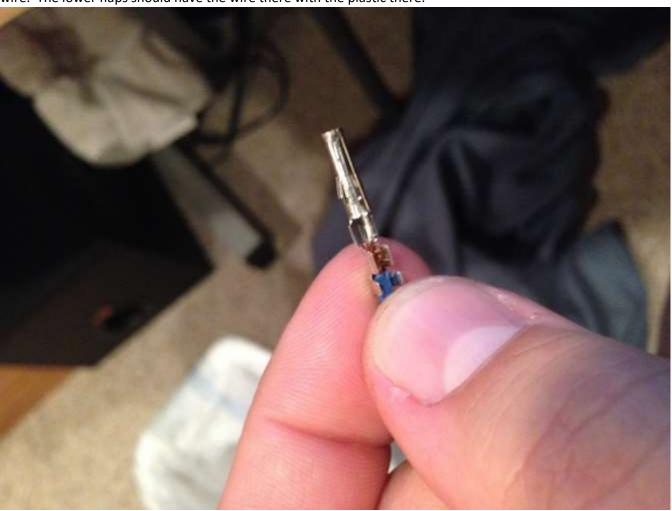
Now using a pliers (or the pliers on your stripper/crimper tool) you will be carefully folding over one flap at time around the copper wire.
