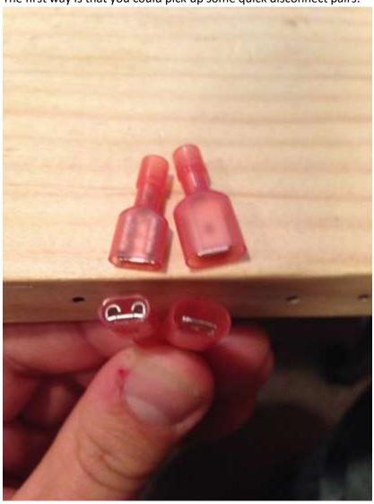
As you can see, one end is a quick disconnect like you are familiar with. The other connector is a spade like connector which slides into the other. So it just joins the two wires that way. This way is nice because you are familiar with stripping and quick disconnects already. You only need to do this on one side of the fuse holder, so that it's attached to the live wire from the CP. I don't think I told you to buy these quick disconnect pairs, but they should sell them at hardware stores.
